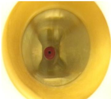
Internal chamber of the latex stomach before adding milk and SGF (Simulated Gastric fluid).
