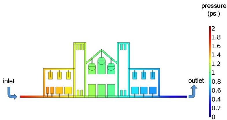
Figure S4. Simulation of pressure distribution inside a microfluidic network. The flow direction is from left to right.
