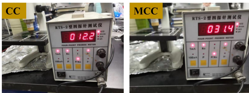
Fig. S8. Four-point probe method for measuring square resistance of CC and MCC.
