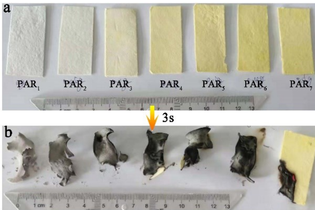
Figure S2 (a) PAR 1-7 (long ~ 4.5 cm, width ~ 1.5cm) (b) The tweezers clamped PAR 1-7 and ignited in the flame of the flame for 3 s, then moved away from the embers that allowed it to burn naturally in the air.
