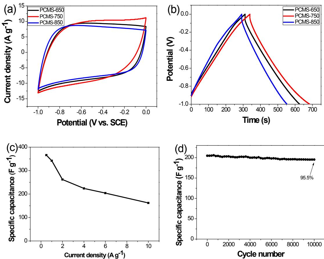
Figure S1: CV curves of PCMS-T at  $5 \text{ mV s}^{-1}$  in  $0.5 \text{ M Na}_2\text{SO}_4$  aqueous solution (a); GCD curves of PCMS-T at  $1 \text{ A g}^{-1}$  in  $0.5 \text{ M Na}_2\text{SO}_4$  aqueous solution (b); Specific capacitances of PCMS-750 at different current densities in  $0.5 \text{ M Na}_2\text{SO}_4$  aqueous solution (c); Cycling stability of PCMS-750 at  $6 \text{ A g}^{-1}$  in  $0.5 \text{ M Na}_2\text{SO}_4$  aqueous solution (d).
