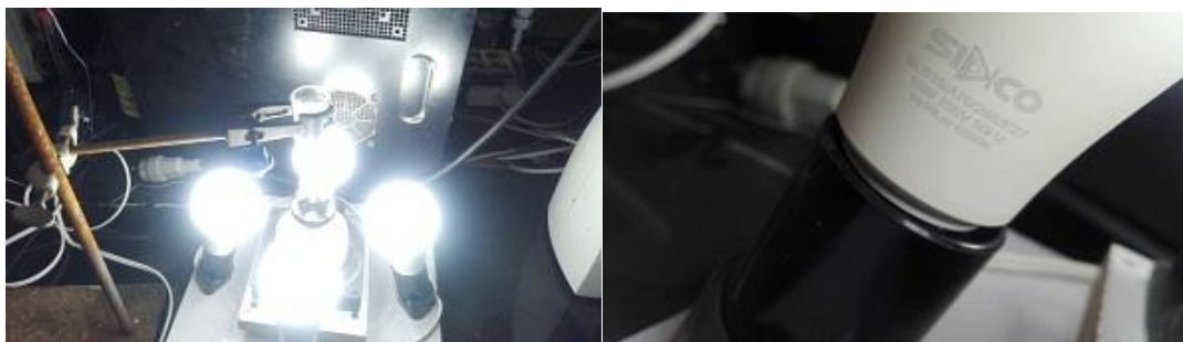
Figure 10. Gram scale photocatalytic system with 16W Fluorescent lamp
