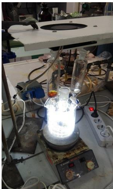
Figure 12. Gram scale photocatalytic system with 5 W white LED and dropping flow
