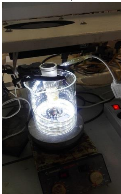
Figure 9. Gram scale photocatalytic system with 5 W white LED
