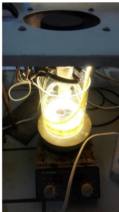
Figure 11. Gram scale photocatalytic system with 5W Sun light LED
