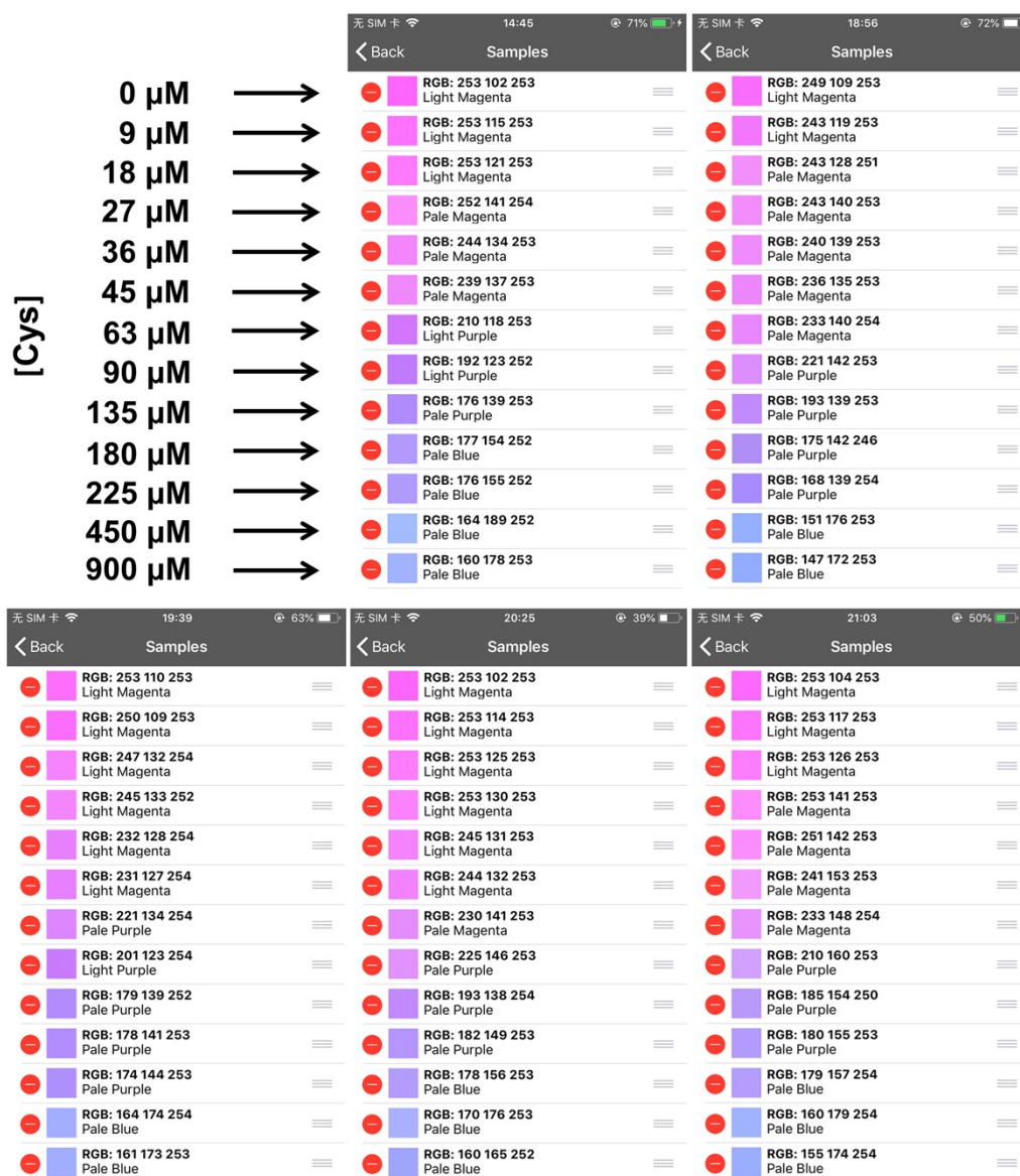
Fig. S13. The RGB values of smartphone-based analysis for detecting Cys in the release capsule by probe Sm-2 n impregnated test paper strips with five repetitions.
