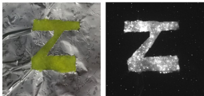
Figure S6 Optical and X-ray image of \text{CsPbBr}_3/\text{Cs}_4\text{PbBr}_6 powder that record by CCD camera. X-ray image excited with 40keV X-ray.
