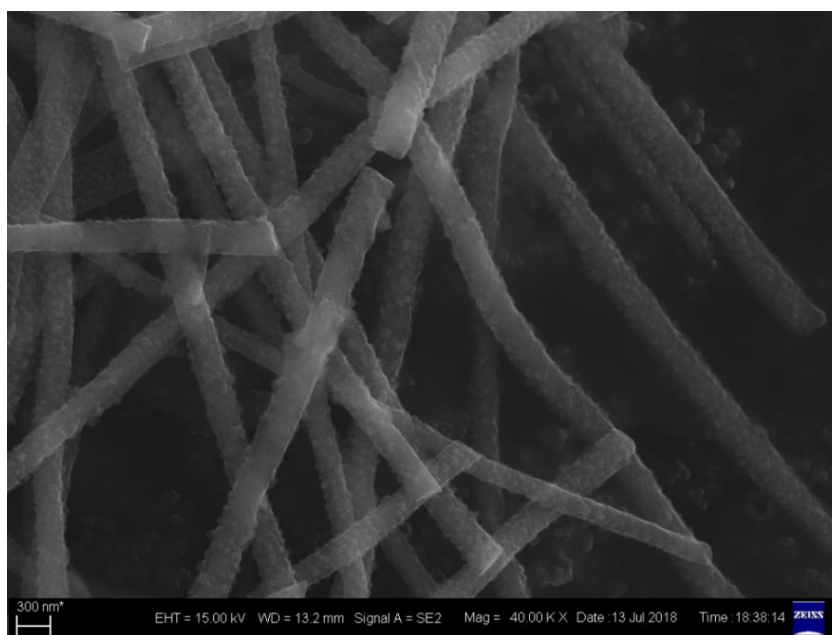
Figure S27 SEM image of the NiCo 2 -N 3 -S 3 -C after chronopotentiometry measurement.
