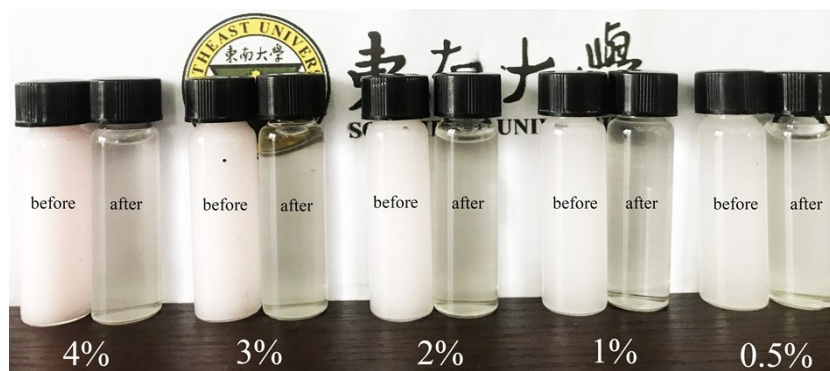
Fig. S4. Images of emulsions with different initial oil content before and after separation using PG-MS.
