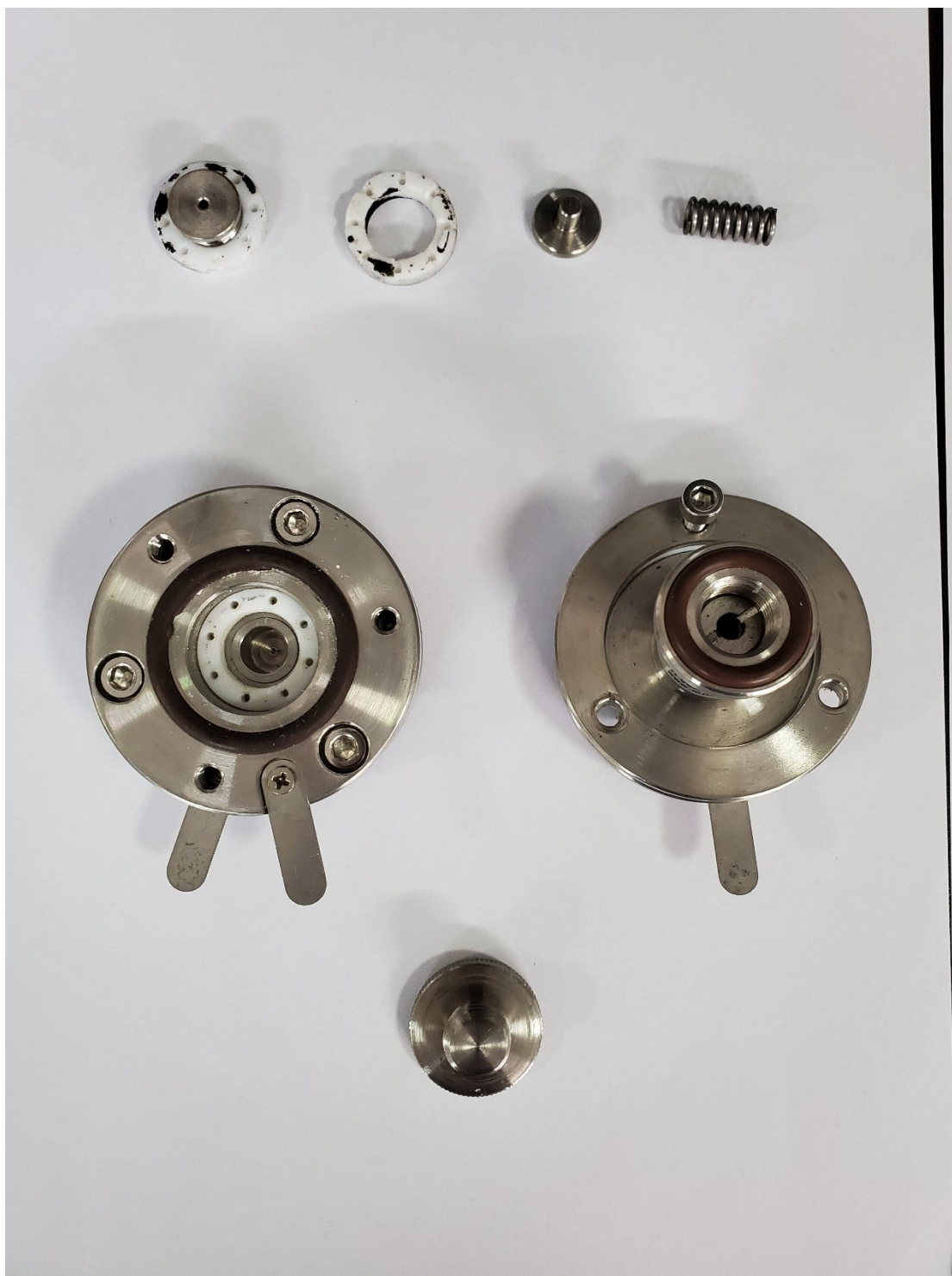
Figure S2 Digital photo of removable three-electrode battery.
