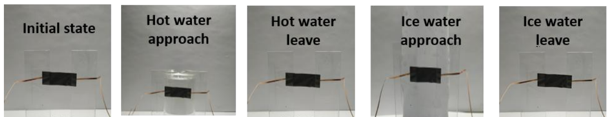
Figure. S10. Optical photos of the tests for the CNT-MC film as a temperature sensor.
