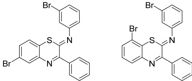
The reaction was conducted with acetophenone (**1a**, 47 μL, 0.4 mmol), 3-bromoaniline (**2k**, 44 μL, 0.4 mmol) and S (25.6 mg, 0.8 mmol). The residue was purified by column chromatography on silica gel (petroleum ether/EtOAc: 200/1) to yield the desired product **4j+4j'** (48.9 mg, 52%) as yellow solid. mp: 149–150 °C, 114–115 °C.
