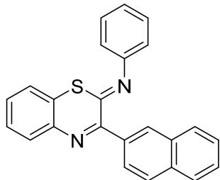
The reaction was conducted with 1-(naphthalen-2-yl)ethan-1-one (**1w**, 69 mg, 0.4 mmol), aniline (**2a**, 37 μL, 0.4 mmol) and S (25.6 mg, 0.8 mmol). The residue was purified by column chromatography on silica gel (petroleum ether/EtOAc: 200/1) to yield the desired product **3w** (19.7 mg, 27%) as yellow solid. mp: 175–176 °C.
