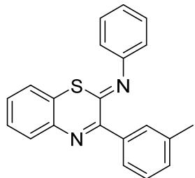
The reaction was conducted with 1-(m-tolyl)ethan-1-one (**1k**, 54  $\mu$ L, 0.4 mmol), aniline (**2a**, 37  $\mu$ L, 0.4 mmol) and S<sub>8</sub> (25.6 mg, 0.8 mmol). The residue was purified by column chromatography on silica gel (petroleum ether/EtOAc: 200/1) to yield the desired product **3k** (39.4 mg, 60%) as orange solid. mp: 140-141 °C.
