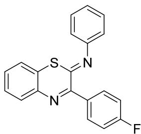
The reaction was conducted with 1-(4-fluorophenyl)ethan-1-one (**1e**, 49  $\mu$ L, 0.4 mmol), aniline (**2a**, 37  $\mu$ L, 0.4 mmol) and S (25.6 mg, 0.8 mmol). The residue was purified by column chromatography on silica gel (petroleum ether/EtOAc: 200/1) to yield the desired product **3e** (42.5 mg, 64%) as yellow solid. mp: 117-118 °C.
