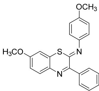
The reaction was conducted with acetophenone (**1a**, 47  $\mu$ L, 0.4 mmol), 4-methoxyaniline (**2e**, 50 mg, 0.4 mmol) and S (25.6 mg, 0.8 mmol). The residue was purified by column chromatography on silica gel (petroleum ether/EtOAc: 20/1) to yield the desired product **4d** (29.9 mg, 40%) as yellow solid. mp: 131-132 °C.
