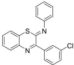
The reaction was conducted with 1-(3-chlorophenyl)ethan-1-one (**1m**, 53  $\mu$ L, 0.4 mmol), aniline (**2a**, 37  $\mu$ L, 0.4 mmol) and S (25.6 mg, 0.8 mmol). The residue was purified by column chromatography on silica gel (petroleum ether/EtOAc: 200/1) to yield the desired product **3m** (49.4 mg, 71%) as orange solid. mp: 92-93 °C.
