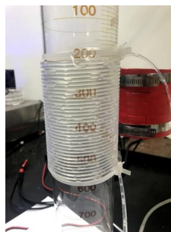
layout of the inlet and outlet PFA tube (For clarity, solvent only, no catalysts and indole in the above two photos)
