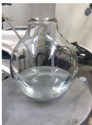
layout of the inlet and outlet PFA tube (For clarity, solvent only, no catalysts and indole in the above two photos)
