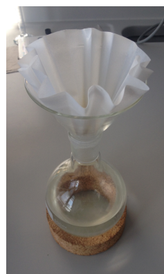
d) Filtration of the reaction mixture
