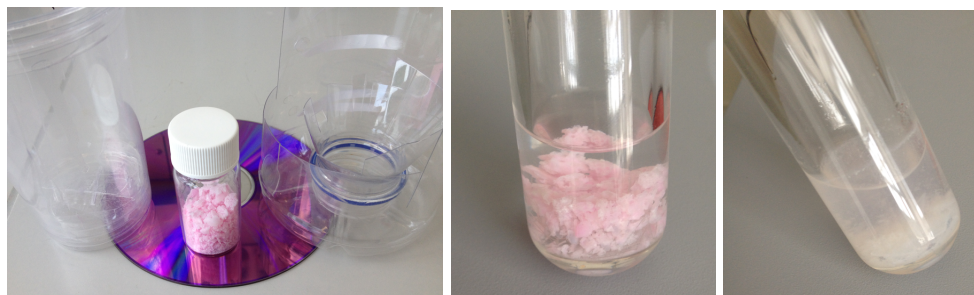
Figure S7. Left: PLA transparent cup; 4 isolated from a DVD; PET transparent bottle. Middle: Reaction mixture before microwave heating. Right: Reaction mixture after microwave heating.
