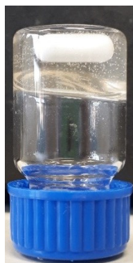
Figure S9 Highly viscous polyacrylamide solution obtained after 3 min of reaction (Exp 14).
