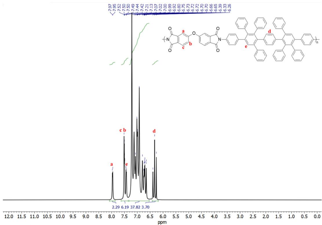
Figure S6.  $^1\text{H}$  NMR (500 MHz,  $\text{CDCl}_3$ ) spectrum of PAPI 4.
