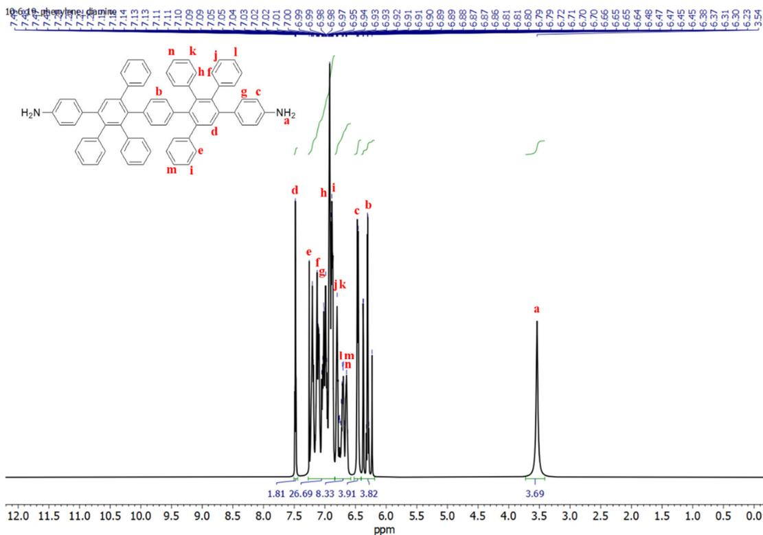
Figure S1.  $^1\text{H}$  NMR (500 MHz,  $\text{CDCl}_3$ ) spectrum of phenylated phenylenediamine.
