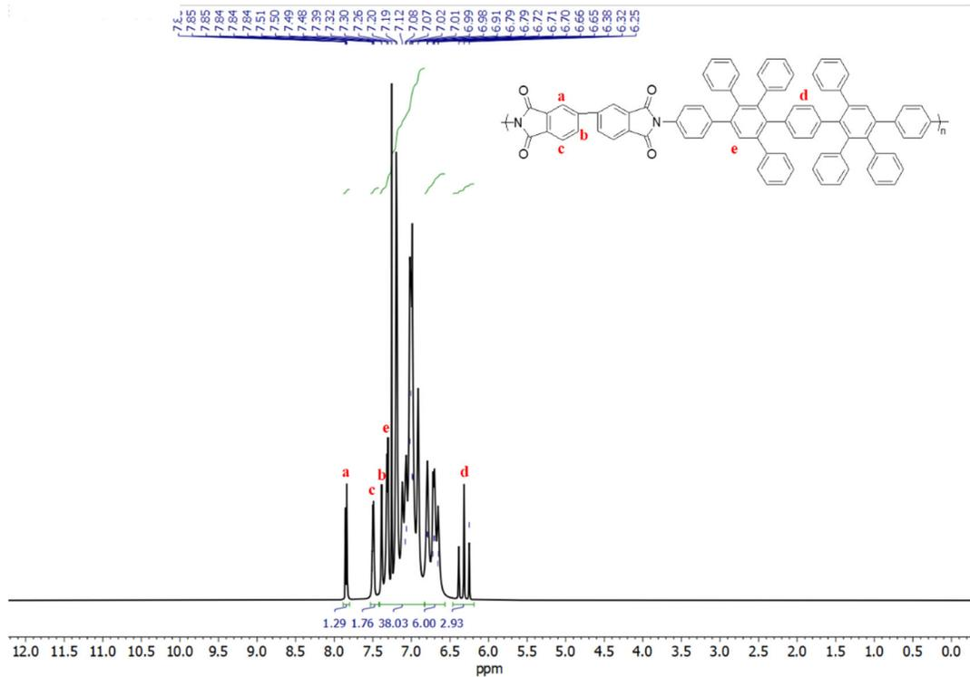
Figure S4.  $^1\text{H}$  NMR (500 MHz,  $\text{CDCl}_3$ ) spectrum of PAPI 2
