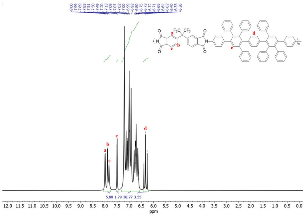
**Figure S7.**  $^1\text{H}$  NMR (500 MHz,  $\text{CDCl}_3$ ) spectrum of PAPI 5.
