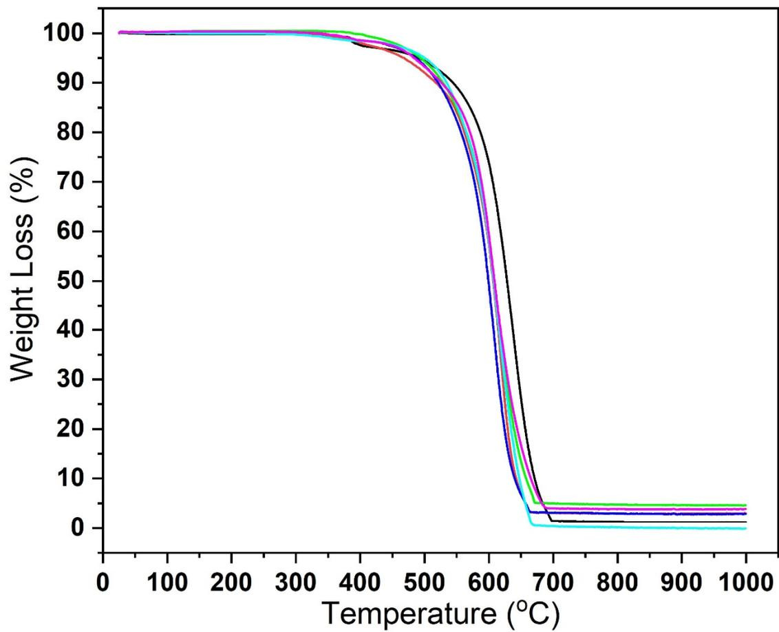
**Figure S11.** Thermal gravimetric analysis (TGA) results of PAPI 1-6 using a heating rate of 10 °C/min and under an atmosphere of air.
