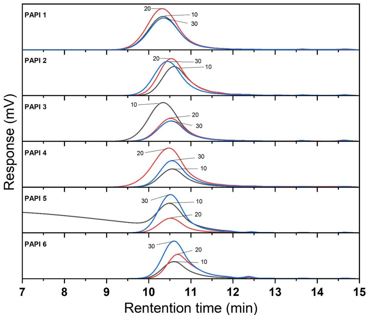
**Figure S10.** Gel permeation chromatography (GPC) results for PAPI 1-6 at 10, 20, and 30 min; 4 columns at 40 °C, HPLC-grade THF at a flow rate = 0.35 mL/min, polymer sample concentration = 1 mg/mL filtered through 0.2- $\mu$ m PTFE syringe filter, refractive index detector, and calibration based on linear polystyrene standards.
