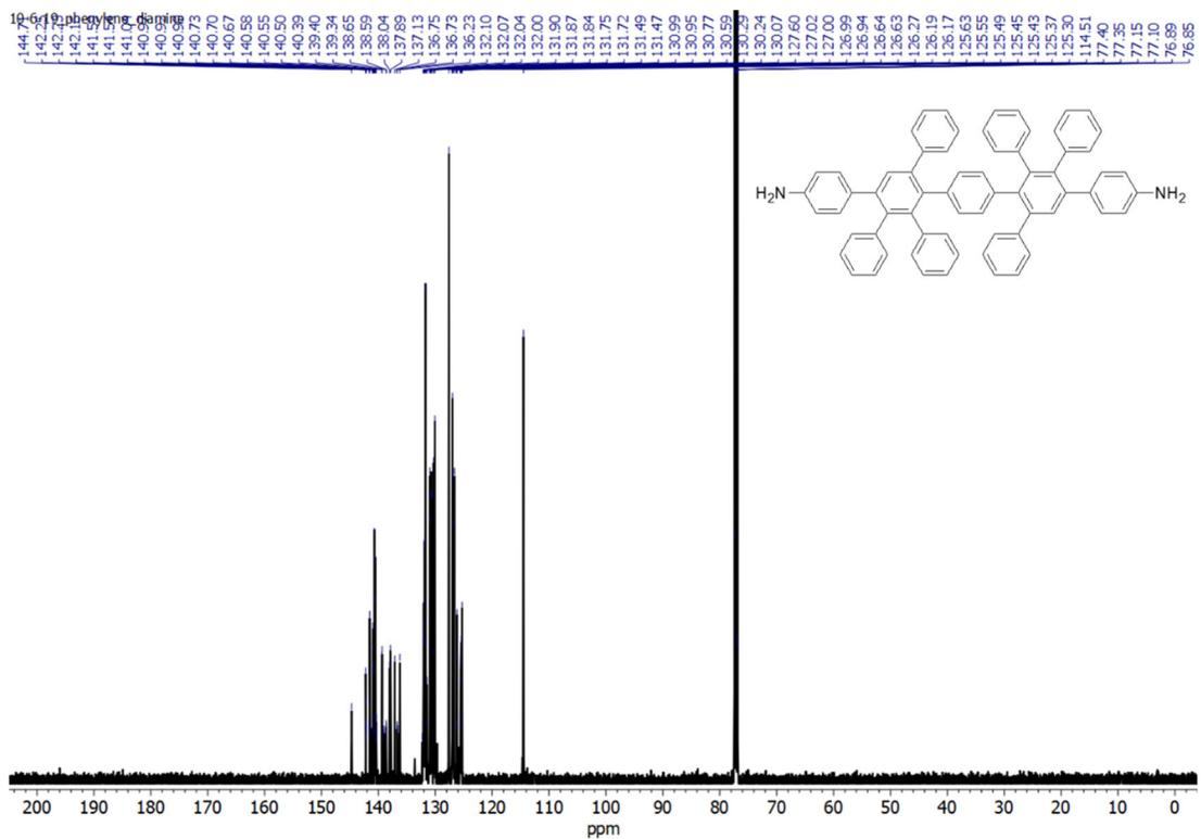
Figure S2.  $^{13}\text{C}$  NMR (125 MHz,  $\text{CDCl}_3$ ) spectrum of phenylated phenylenediamine.
