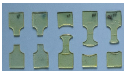
Figure S5. Photograph of self-healed P1 samples (120 °C, 4 h) after tensile experiment, which did not break at the repair sites.
