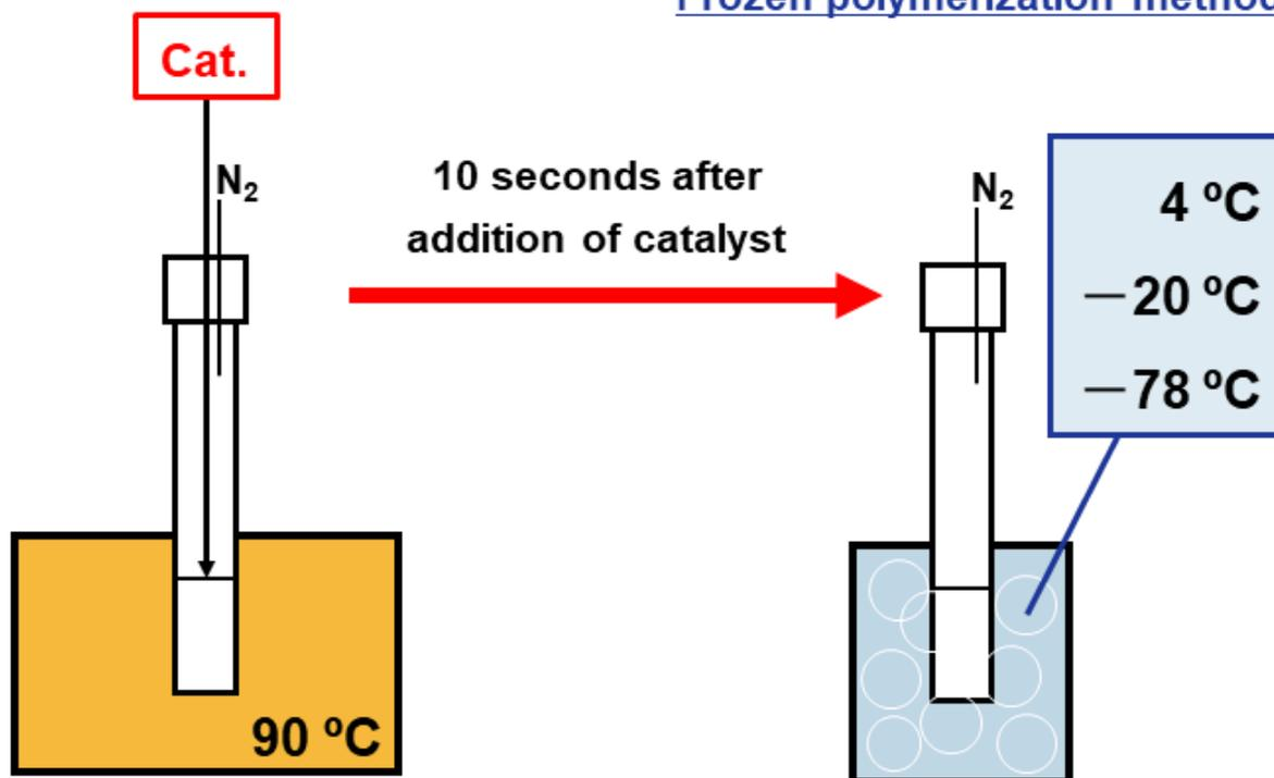
**Figure S1.** The experimental method of "frozen polymerization".
