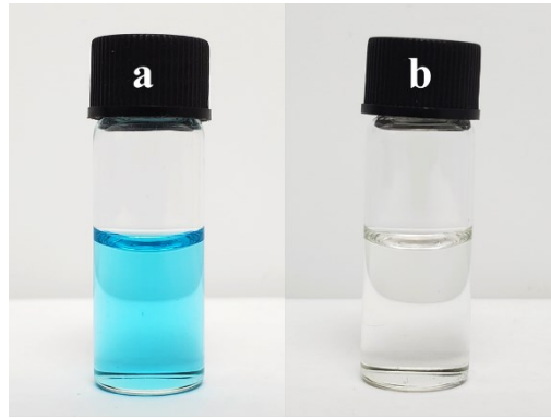
Figure S10. (a) \text{Cu}^{2+} crosslinked \text{cP4VP}_{60\text{k}} dispersion in DMF and (b) after feeding EDTA and dialysis.
