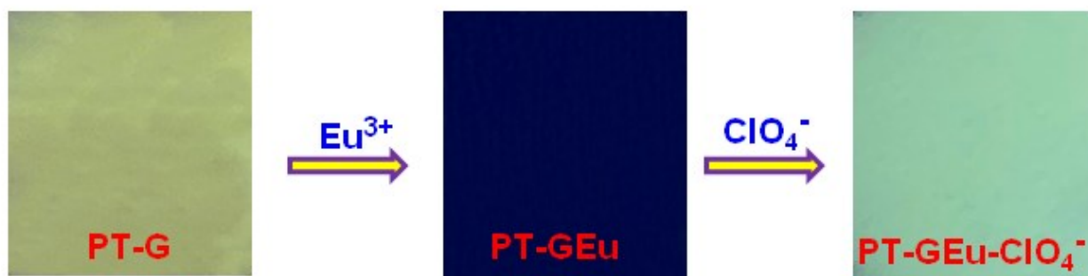
Figure S33. Fluorescence colors changes (under the UV lamp, at \lambda_{\text{ex}} = 365 \text{ nm} ) of the PT-G and PT-GEu -based test kits after addition of different concentration \text{Eu}^{3+} and \text{ClO}_4^- (from 0 M to 0.1 M).
