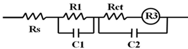
Fig. S11 Equivalent circuit used to fit the impedance measurements on the DSSCs.
