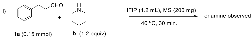
Scheme S9: Enamine formation of 1a with b in HFIP solvent
