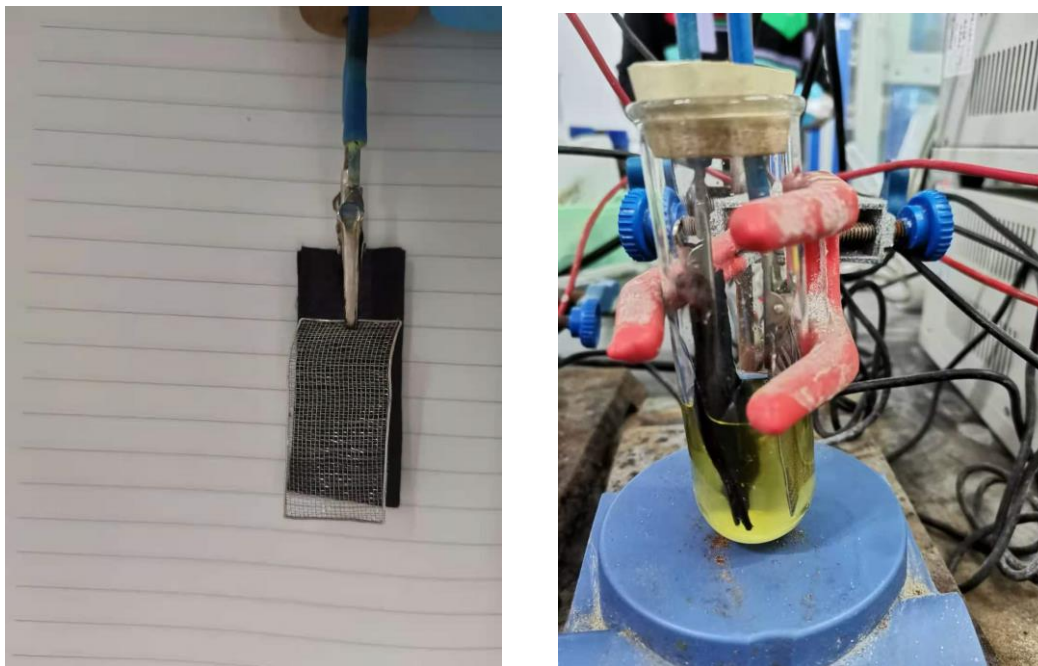
Figure S2. Gram-scale electrolysis setup (carbon cloth: width 2.5 cm, immersion depth 3 cm; platinum gauze electrode: width 2.5 cm, immersion depth 3 cm)
