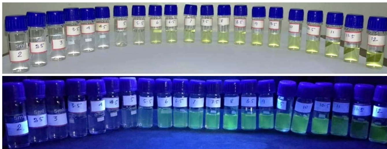
Fig. s15 Colors of HM-2py-B in the presence of different pH media under visible light (upper row) and UV light (lower row) in Britton Robinson buffer at room temperature.
