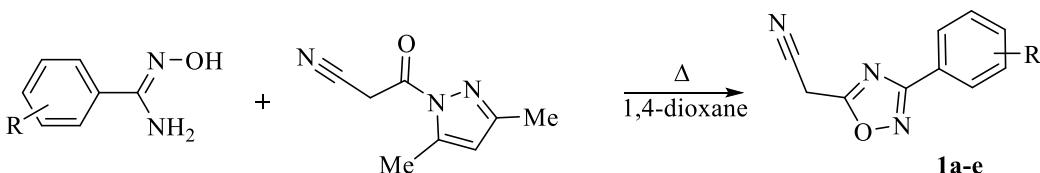
A mixture of equimolar amidoxime (10 mmol) and 3-(3,5-dimethyl-1*H*-pyrazol-1-yl)-3-oxopropanenitrile (1.63 g, 10 mmol) in 25 ml of dioxane was refluxed for 24 hours. Then cooled and dioxane was evaporated in vacuum. The residue was washed with  $\text{NaHCO}_3$  solution, filtered and dried yielding the target (1,2,4-oxadiazol-5-yl) acetonitrile 1.
