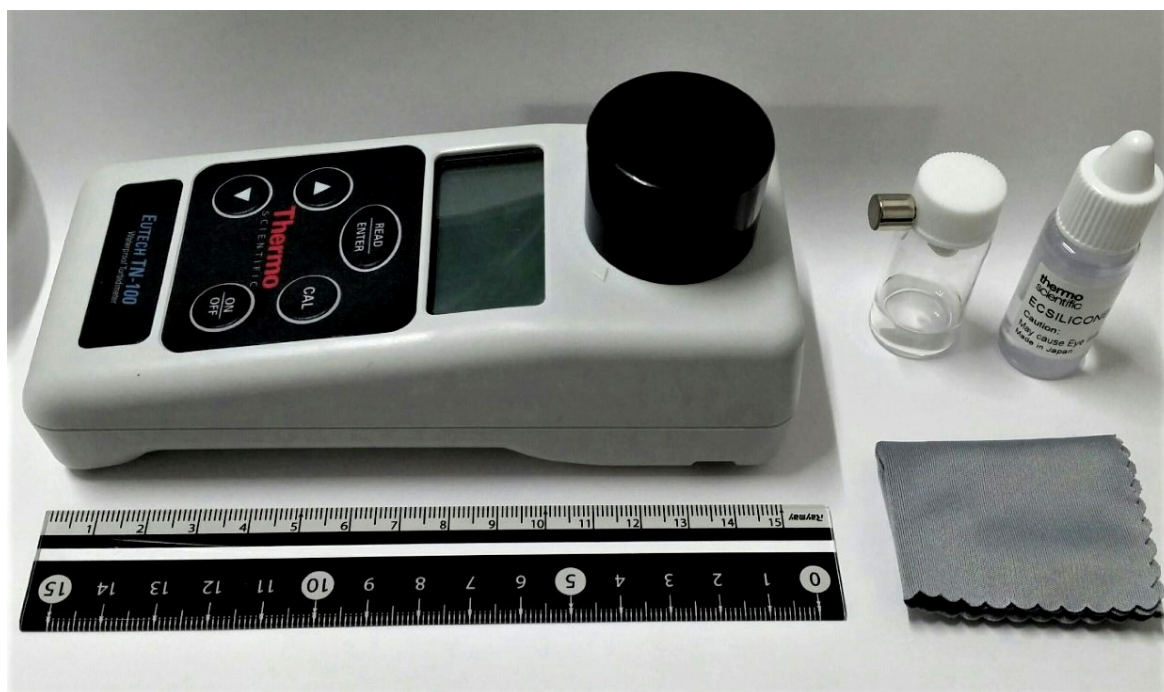
Figure S1 Photograph of a turbidity meter with glass vial (the stirrer bar is fixed with a magnet), silicone oil and a cloth.
