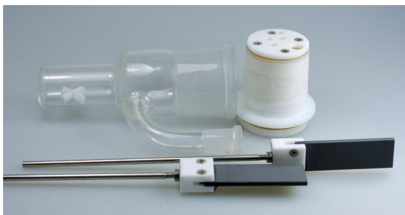
Figure S2: 25 mL beaker-type electrolysis cell; size of electrodes: 3 mm x 20 mm x 60 mm (not the final electrode materials shown).
