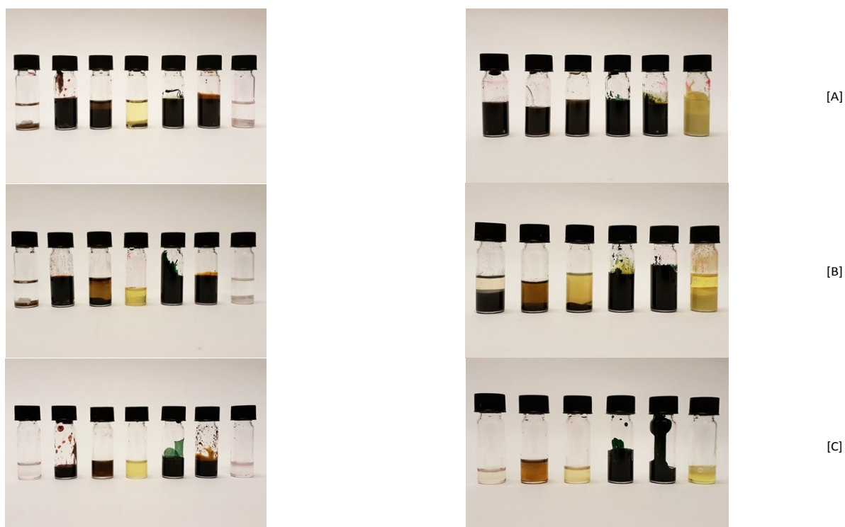
Figure S 12. Metal dissolution process in ChCl:DTT (1:3). [A] Photo after ~24h after beginning the dissolution process, [B] Photo of the centrifuged sample after 48h [C] Photo of the filtrate. From left to right: CdO, CoO, LiCoO 2 , Cu 2 O, Fe 3 O 4 , NiO, ZnO, AgO, Au 2 O 3 , CuO, FeO, Fe 2 O 3 , PbO. Pictures were taken after equilibration at room temperature.
