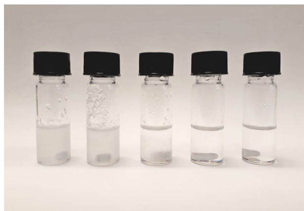
Figure S 2 Mixtures of choline chloride with thioglycolic acid. From left to right the choline chloride to thioglycolic acid molar ratio changes (3:1, 2:1, 1:1, 1:2, 1:3). The picture was taken after equilibration at room temperature.
