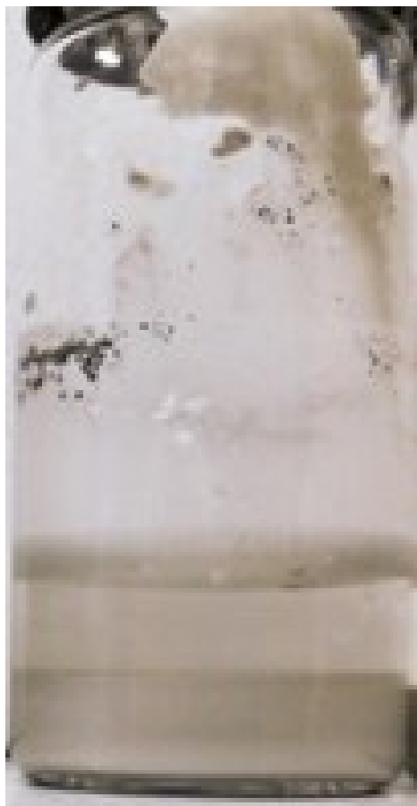
Figure S7. Adsorption of the MXenes physically ( not covalently) grafted with poly(DMAPS- co -AA) onto 4 g of \leq 10\mu\text{m} \alpha\text{-Al}_2\text{O}_3 (BET surface area of 2.32\text{ m}^2\text{ g}^{-1} ) in API brine.
