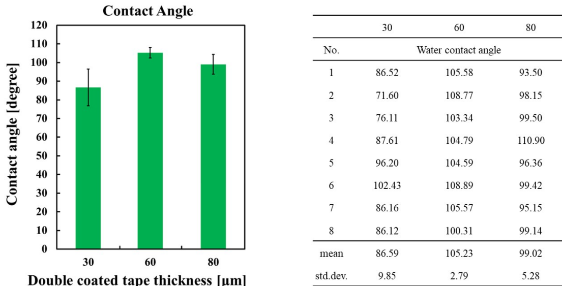
Fig. S1 The water contact angle of 30, 60, and 80 \mu m 8000 series 3M double-side tapes. Error bars obtained from 8 individual measurements
