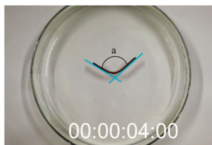
Figure S6. Schematic of angle measurement of a U-shaped PVA/TP hydrogel during shape recovering.
