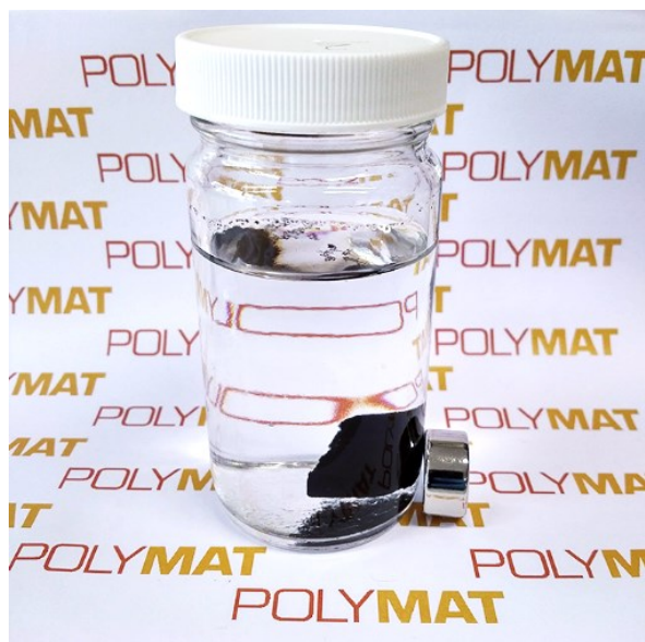
Fig. S2 The 3D rGO@Fe 3 O 4 structure in the aqueous solution and in the presence of an external magnet.
