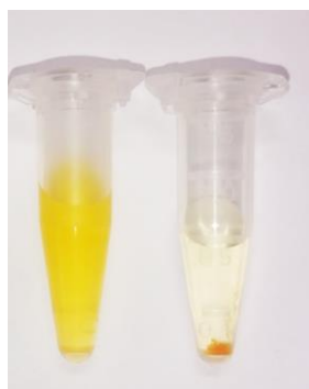
Figure S3. Nanoparticles dispersed in aqueous solution containing sodium phosphate buffer (5 mM, pH 7.0). Left: Nanoparticles with phosphonate groups on their external surface (pM-Ru). Right: Nanoparticles without phosphonate groups on their external surface (M-Ru).
