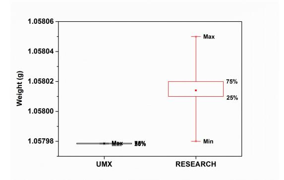
Fig. A.2 The box-plot of the substrate weight measured with the UMX and RESEARCH balancesis formed from the minimal and maximal value (whiskers), values of 25th and 75th percentil and the arithmetic mean (solid square in the box).
