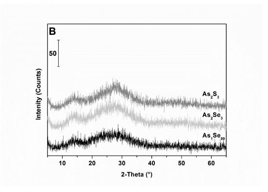
Fig. A.1 XRD of As<sub>2</sub>S<sub>3</sub>, As<sub>2</sub>Se<sub>3</sub> and As<sub>1</sub>Se<sub>99</sub> bulk glasses (A) and the corresponding thin films (B).
