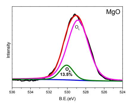
**Figure S1.** The O 1s XPS spectrum of MgO NPs.
