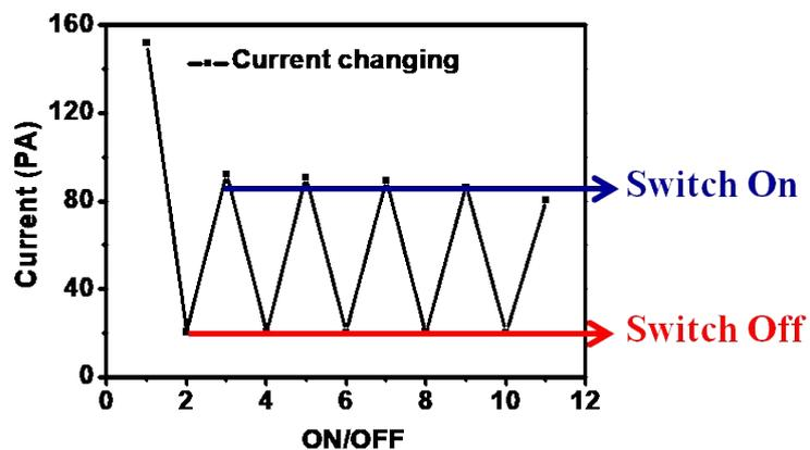
Figure S5. The reversible single-molecule ligand-gating switch could be operated five times and the current recordings could maintain about 80-90 pA and  $\sim$ 20 pA under switch on/off state.
