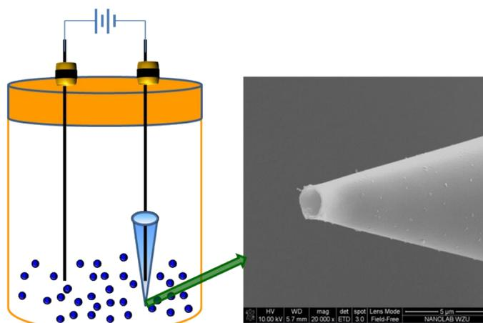
Figure S3. Picoammeter for current testing (left) and SEM image of nanocapillary after stretching (right).
