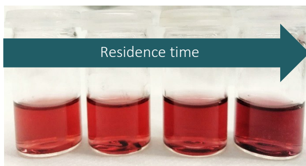
Figure S14. Impact of the residence time on the preparation of Au NPs
