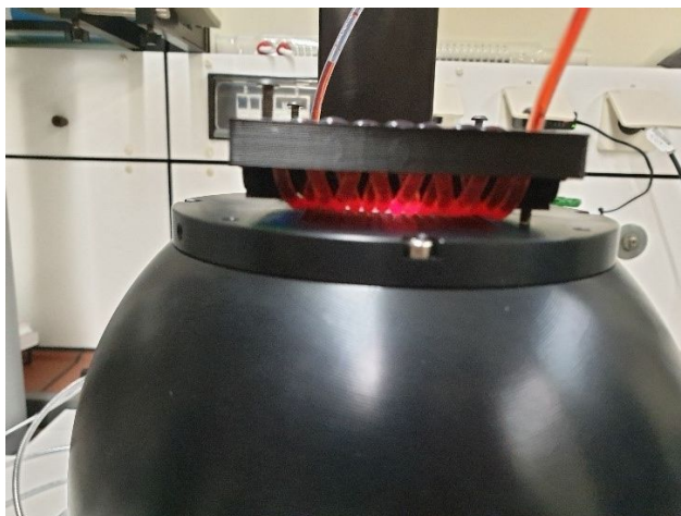
Figure S11 Picture of the SR reactor, positioned over the sample port of the integrating sphere. The top part of the reactor, holding the capillaries in place was removed to allow positioning of the capillaries directly on the sample port.
