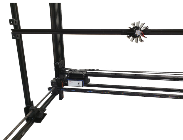
Figure S2 Picture of a part of the scanning device, illustrating how objects are mounted on the z-carriage.
