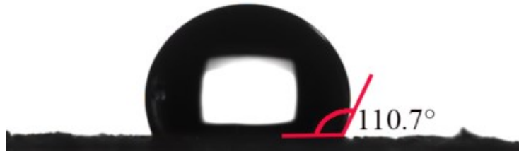
Figure S1 The water contact angle measurement of industrial \text{Fe}_3\text{O}_4 -por after cycling test
