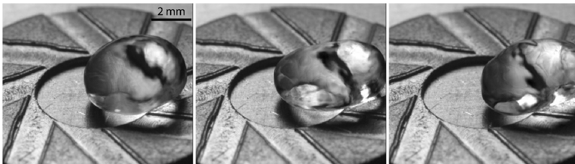
Figure S9. Leidenfrost droplet leaning on the edge of the disk during the self-propulsion mode, which enables it to hover on the top surface of the disk.
