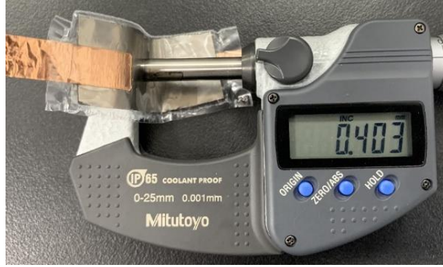
Fig. S13 Photograph of measuring the thickness of a thin-film PVA/G Zn// \delta -MgVO battery with a micrometer caliper.
