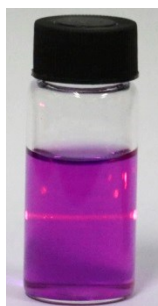
Fig. S3. Digital photograph of a ZIF-67 suspension in ethanol with Tyndall effects.
