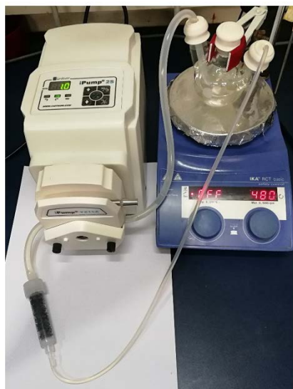
Figure S23. The image of the continuous-flow setup for PCB 77 degradation.
