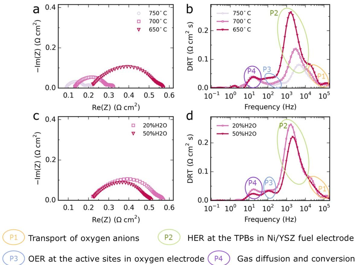
**Fig. S5** EIS data on Ni/YSZ fuel-electrode-supported cells with the hybrid-coated LSF oxygen electrode measured under OCV conditions. Effects of temperature on the EIS data recorded with 20% $\text{H}_2\text{O}$ -80% $\text{H}_2$  fed to the fuel electrode and dry air to the oxygen electrode. (a) Nyquist plots and (b) DRT plots. Effects of steam content in the fuel electrode on the EIS data recorded at 650 °C. (c) Nyquist plots and (d) DRT plots.
