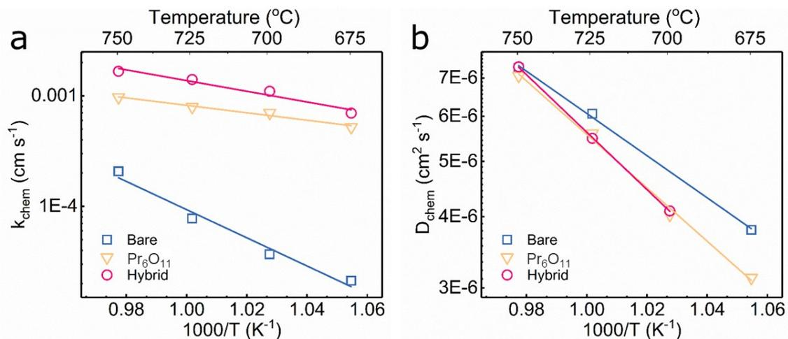
**Fig. S2** (a) Surface exchange coefficient ( $k_{\text{chem}}$ ) and (b) chemical diffusion coefficient ( $D_{\text{chem}}$ ) of the bare LSF, Pr<sub>6</sub>O<sub>11</sub>-coated LSF, and hybrid-catalyst-coated LSF electrodes obtained from the ECR measurements.
