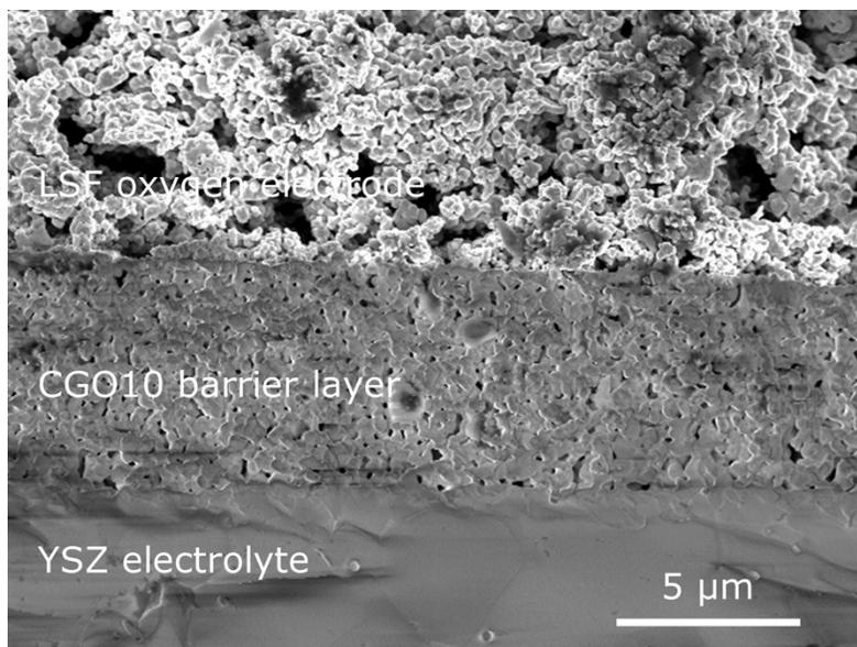
**Fig. S4** Cross-sectional SEM image of fuel-electrode-supported cell showing a porous CGO10 barrier layer.
