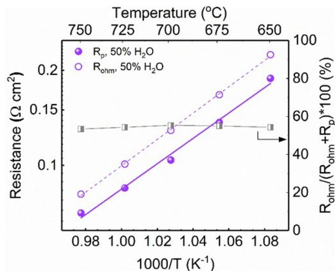
**Fig. S6**  $R_p$  and  $R_{ohm}$  plotted as a function of inverse temperature, measured on the double-side modified cell (with the CGO20-coated Ni/YSZ fuel electrode and the hybrid-catalyst-coated LSF oxygen electrode) with 50% $H_2O$ -50% $H_2$  fed to the fuel electrode and dry air to the oxygen electrode.
