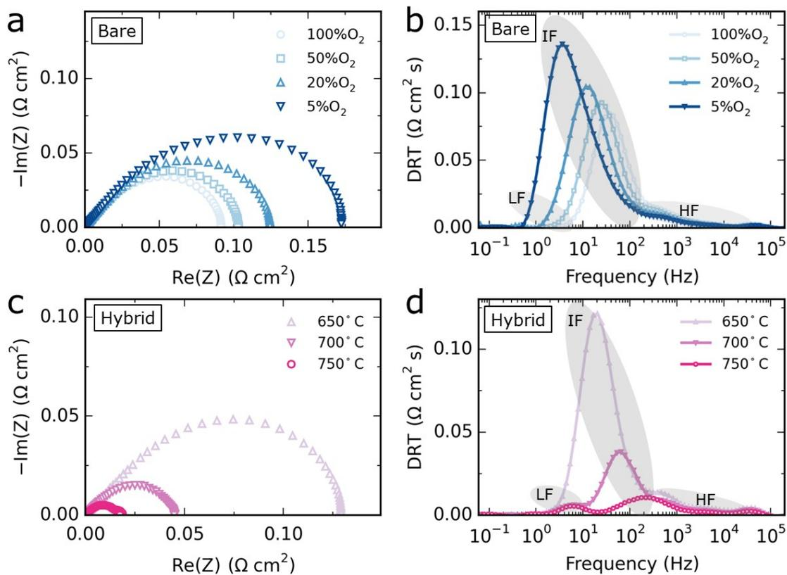
**Fig. S1** Electrochemical performance on symmetrical cells. Effects of oxygen partial pressure ( $p\text{O}_2$ ) on the EIS data of bare LSF electrodes at 750 °C. (a) Nyquist plots and (b) DRT plots. Effects of temperature on the EIS data of hybrid modified LSF electrodes in dry air. (c) Nyquist plots and (d) DRT plots.
