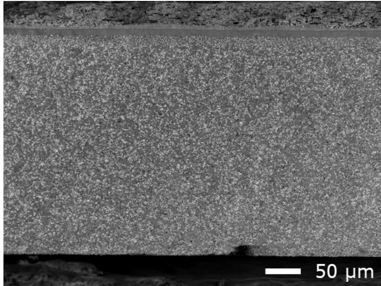
**Fig. S3** Cross-sectional SEM image of fuel-electrode-supported cells with a configuration of Ni/YSZ support | Ni/YSZ fuel electrode | YSZ electrolyte | CGO10 barrier | hybrid-catalyst-coated LSF oxygen electrode (hybrid-catalyst-coated LSF cell).
