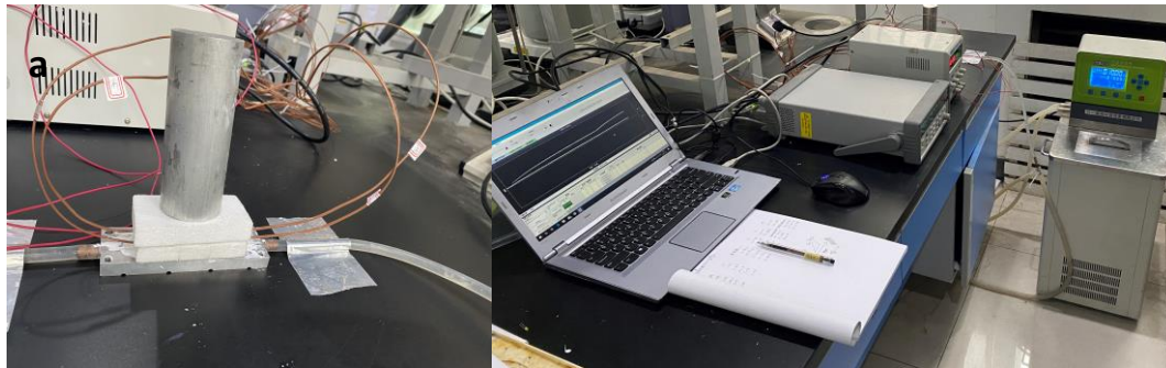
Figure S8 (a) Photograph of thermal conductivity testing platform and (b) schematic illustration of thermal conductivity measurement platform.
