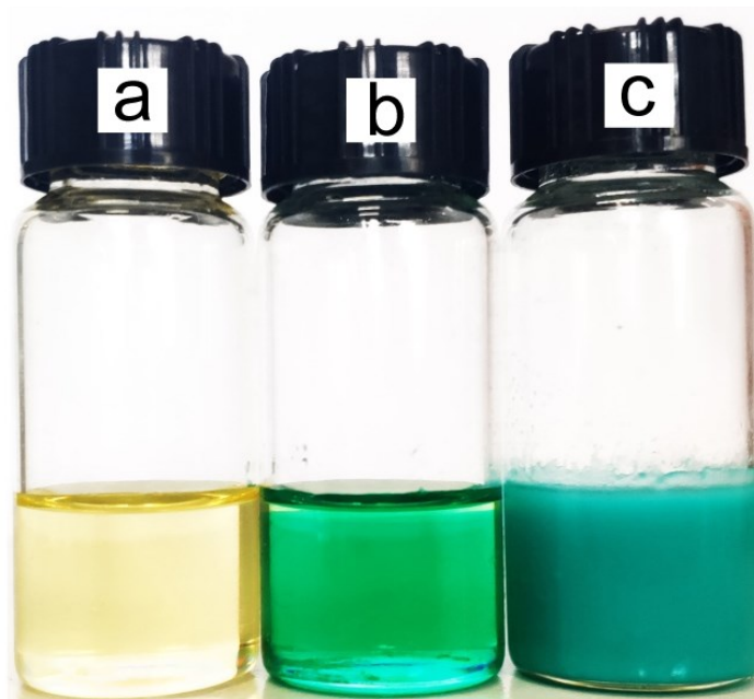
Fig. S1 The color changes of the EMIM-dca IL after addition of \text{Ni}(\text{NO}_3)_2 . (a) Pure EMIM-dca; (b) Mixture of EMIM-dca and \text{Ni}(\text{NO}_3)_2 taken after \text{Ni}(\text{NO}_3)_2 dissolved immediately without stirring; and (c) Mixture of EMIM-dca and \text{Ni}(\text{NO}_3)_2 after stirred overnight.
