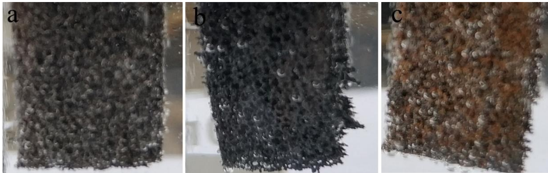
Fig. S30 The images of bubbles on the surface a) FeCO 3 @IF, b) Fe 3 O 4 @IF and c) Fe-O-M@IF during HER process at the current density of 100 mA cm -2
