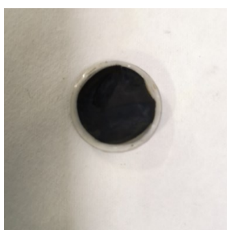
Figure S16 the Optical photo of CNF@V 2 S 3 /S cathode after 500 cycles.
