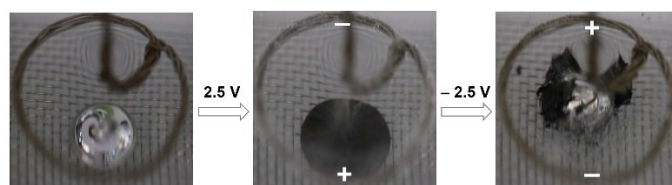
Fig. S2 Electric field adaptive wetting and dewetting of LM droplet on the micro/nanostructured mesh in 1 \text{ mol L}^{-1} KCl solution. The black oxide layer is formed on LM droplet surface when it wets the mesh surface with voltage of 2.5 V. When the voltage of -2.5 V is applied, the black oxide layer will fall off from LM surface, and LM droplet restores to a spherical shape owing to increase of the surface tension.
